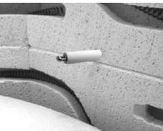
• If the kiln is a manual kiln, it has a *Pyrometric Cone* that is a temperature gauge used to turn the kiln off once it starts melting and drops in the kiln sitter cone supports.
